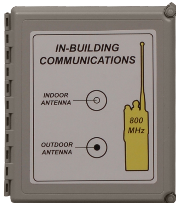
A standard building interface for radio enhancement uses a NEMA 4-type enclosure approximately 10" x 12" in size, is mounted on the building's exterior near the entry point used by emergency personnel, and has standard, conspicuous markings. Enhanced Built-in Solution
